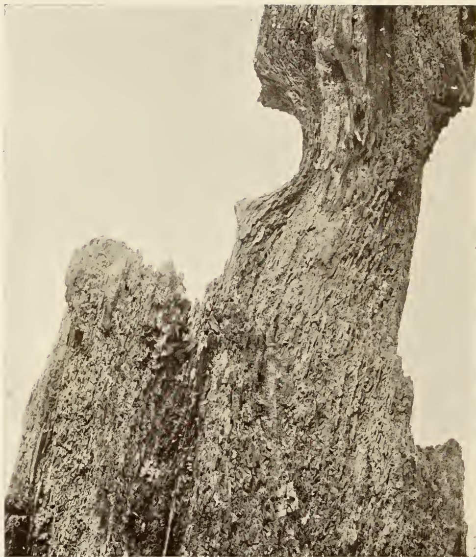
PIECE OF TIMBER FROM RYDE PIER SHOWING DAMAGE CAUSED BY Limnoria AND Chelura (From Brit. Mus. Guide.)
